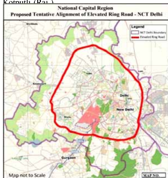
Figure 5.3: Tentative alignments of Elevated Outer Ring Road (EORR)
